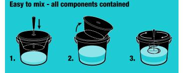
1. Pierce the centre of the lid on the top chamber and push through to pierce the centre of the base also. Allow the material (hardener) to fully drain from the top container into the base. This will normally take between 3 and 5 minutes.
