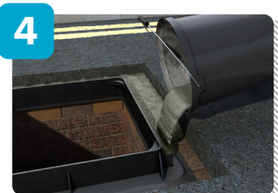
Once the bedding mortar has set, backfill with UltraCrete QC10 F, QC10, Envirobed® CD534 Flowable or PY5.
